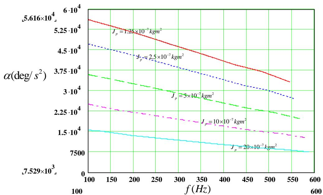
If the motor is running at frequency  $f_o$ , the maximal next frequency you can give is  $f_i$ :
